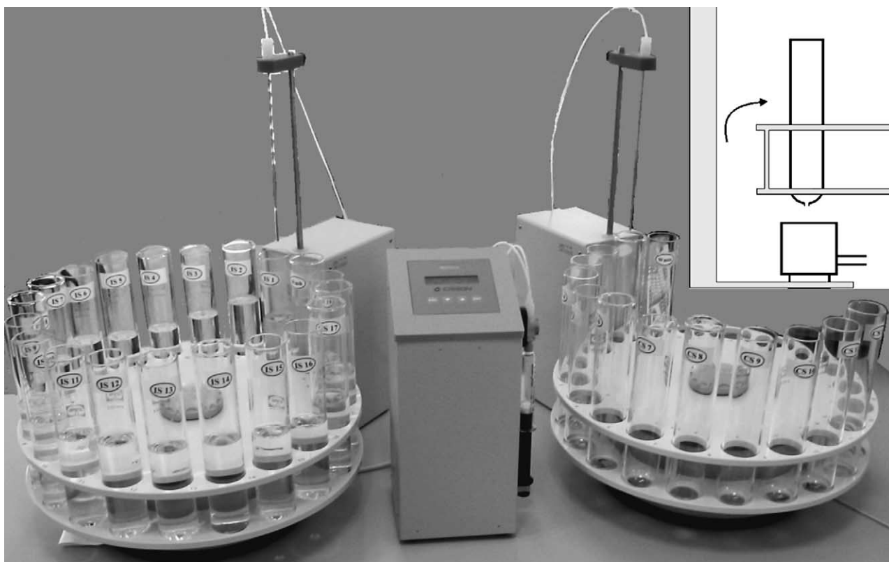
Fig. 1. View of the device used for the automatic sample composition of liquid samples following SSC principles. Upper right part shows a scheme of the drainage tube in sampler 2.
